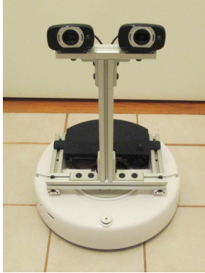
Fig. 4. iRobot Create with Raspberry Pi and webcams
