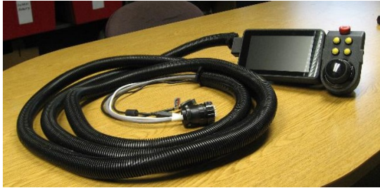
Fig. 4: Open-Source Teach Pendant Prototype [17]
