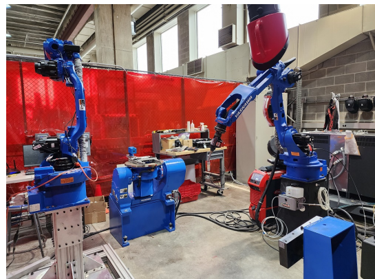
Fig. 2: Robotic WAAM testbed for Convergent Manufacturing [31]
