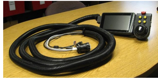
(a) Open-Source Teachpendant Raspberry Pi 4 Prototype
